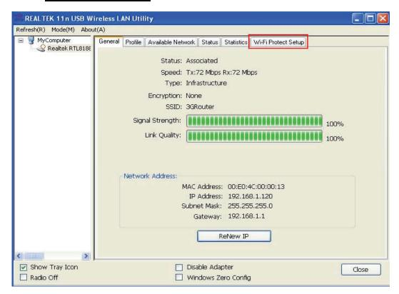
**3.** You can use PIN code or Push-Button configuration, and WPS-compatible wireless access point must use the same type of WPS. For instructions on setup each type of WPS, see next 2 chapters for detailed instructions.
