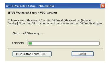
Please activate Push-Button function on wireless access point now, and wireless network card will establish secure connection with access point within one minute.
