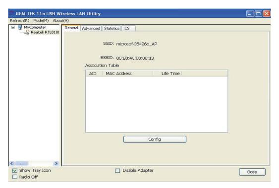
After mode switch is complete, you'll see general information of software AP, which shows AP's SSID and connected wireless clients.
