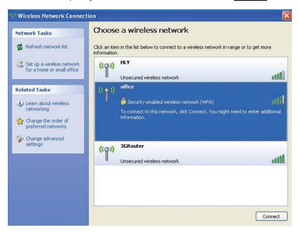
**8.** If the access point is protected by encryption, you have to input its security key or passphrase here. It must match the encryption setting on the access point. If the access point you selected does not use encryption, you'll not be prompted for security key or passphrase.
