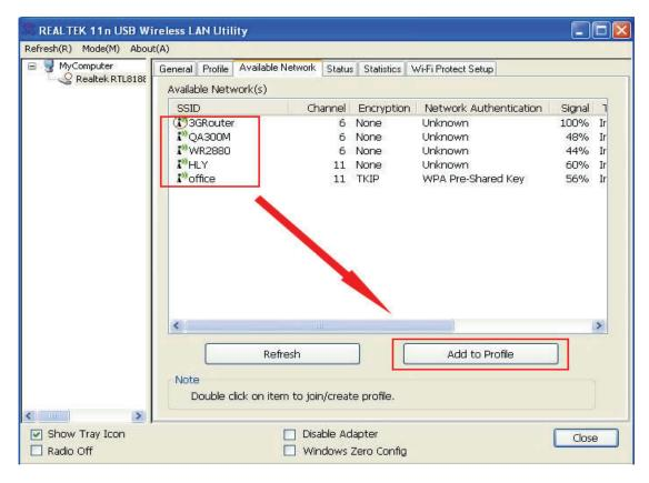
If the wireless access point you wish to connect does not appear here, you can click '**Refresh**' button to scan for wireless access points again; if the wireless access point you're looking for still not appear, try to move the computer closer.
