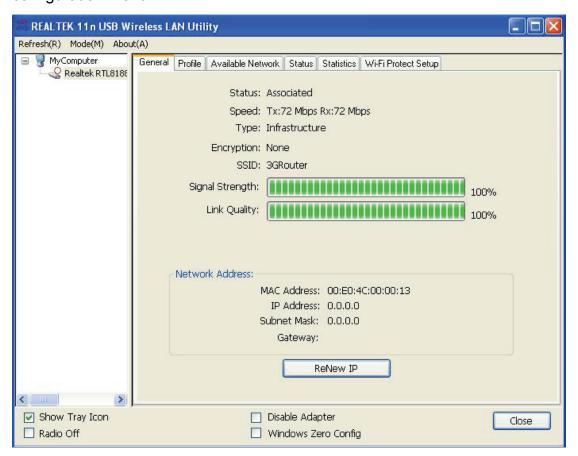
NOTE: If you connected to an access point but the connection has been dropped soon, please check security settings and re-check password spelling.
