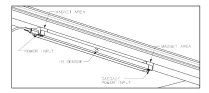
Attention: The power input at the left side is only for cascade powering. If you supply the power from that input (cascade power), IR sensor fuctionality is disabled. The light is immediately activated after the power is On.
