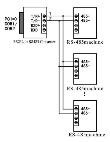
3. half-duplex communication connect between interface converter
